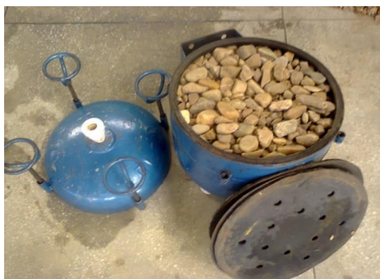
Figure 1. Handcrafted filters using different sizes of gravels and a disc filter
