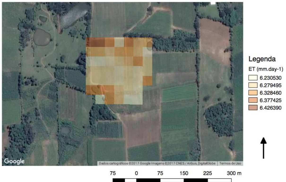
Figure 3. Daily ET obtained from LandSat8 image using METRIC algorithm on 13/jan/2017 over a reference map (Google Images®)
